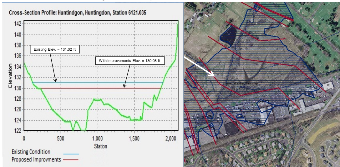
Figure 6.4.C Huntington Valley Creek near Philmont Road, Lower Moreland Twp., Bucks County, PA Modeled Elevation Change with All Improvements in Place = 0.9 ft for 2-Yr Storm Event
