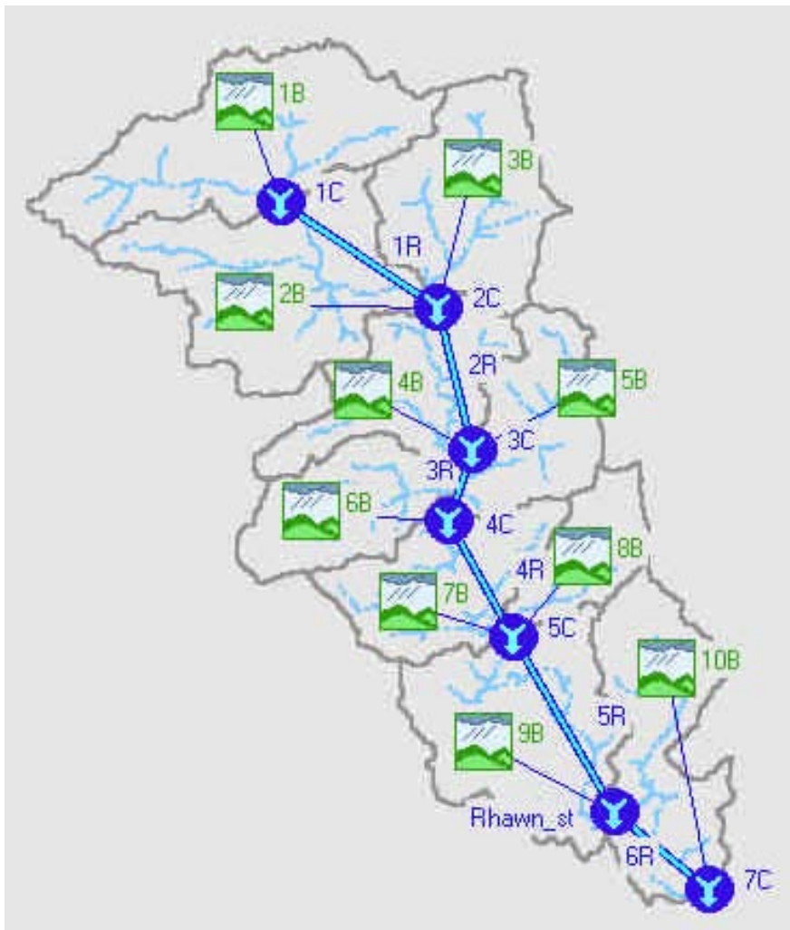
Figure 4.1.A Diagram of Pennypack 10-Subbasin Hydrologic Model used for Flood Insurance Study
