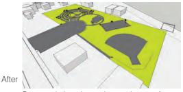
Proposed plan shows the pervious surface decreases to 55 % and impervious surface increases to 45 %.
