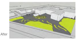
Proposed plan shows 45 % increase in pervious surfaces and the addition of a bioswale and rain garden.
