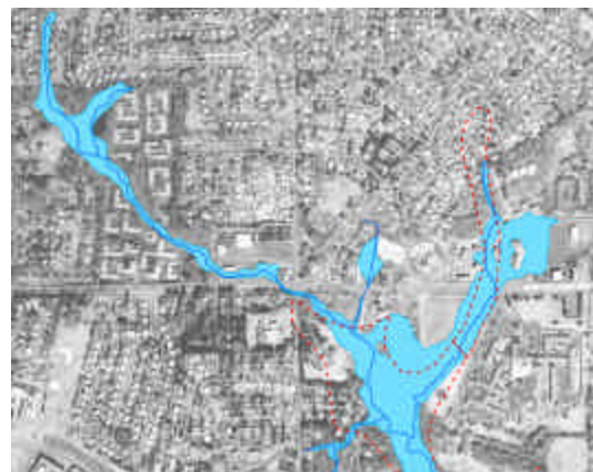
Figure 16: Comparison of 100-year floodplains. Existing boundary is shown in red dotted line and new boundaries are shown as blue areas
