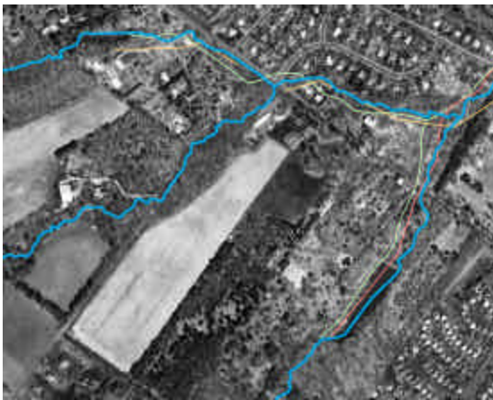
Figure 12: Example of inaccuracy in available stream data in the watershed. Here the blue line represents the accurate stream network, consistent with the ortho-photo. Other available stream files do not match the actual stream location.
